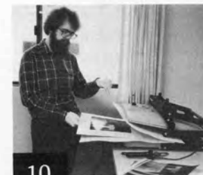
10 Optional method of drying test prints quickly is between pieces of mounting board (reserved for the purpose), heated in a Seal dry-mount press. Only test prints are dried this way.
