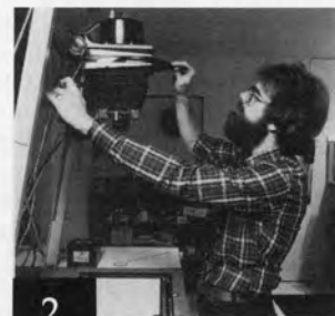
2 Negative receives careful and thorough dusting with a camel's-hair brush. Negative is held at an angle so the dust will fall off.
