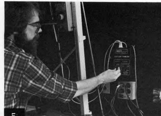
5 Zone VI voltage stabilizer assures constant output of "cold-light" enlarging head. Author prefers this diffused light source for accurate rendition of highlights.
