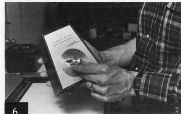
6 Electronic metronome sounds once per second, allowing simple and accurate timing of dodging and burning-in operations, without visual attention.
