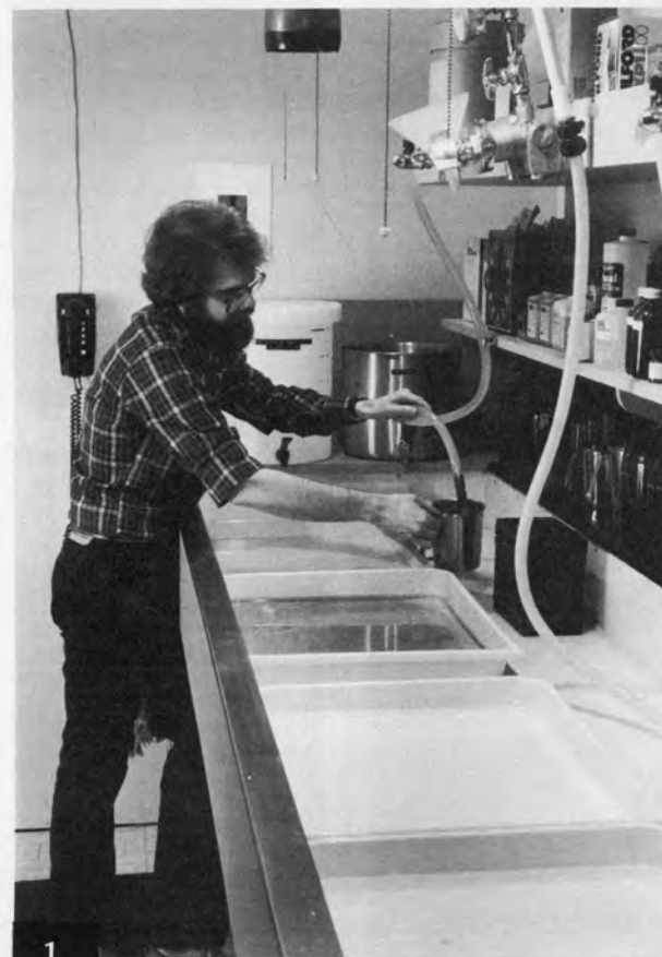
1 Trays are set up for developer (two baths), acetic-acid short stop, first fixer (Kodak F-6 formula with half the recommended hardener), running-water rinse, holding bath. When printing is completed, trays are washed, filled with second fixer, toner, washing aid, and water rinse.
