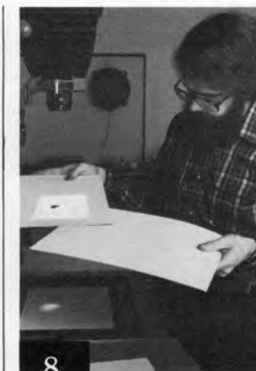
8 Two cardboard sheets are used for burning-in. One has small hole in the center, other is solid, acts as a shutter. Both are white on top for visibility, black on bottom to prevent reflection.
