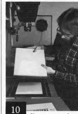
9 Bottom sheet blocks light from reaching paper, ends burning-in of one section.
