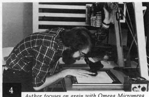
4 Author focuses on grain with Omega Micromega magnifier, resting on a sheet of double-weight enlarging paper. EL Nikkor enlarging lens is then stopped down and rechecked for focus.
