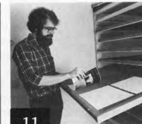
11 Final prints are air-dried on fiberglass screens, in homemade rack. Drying times vary depending on ambient temperature and humidity. Only archivally washed prints are dried here.
