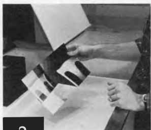
2 Test strip, on Seagull No. 3 paper, is made in three-second steps, ranging from much too light to far too dark. Author uses half sheet of paper, includes highlight areas (to determine exposure) and shadows (to check contrast).
