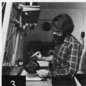
3 Negative in holder is loaded into Beseler 4x5 enlarger. Carrier has been filed out to include the entire image area and a slight surround.
